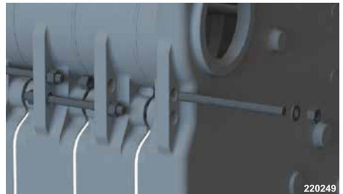
Figure 12 Sealing ring installation and port alignment
